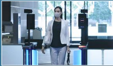
Walk-through facial authentication gates Body surface temperature + face mask detection
